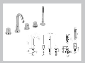
5 hole bath shower mixer deck mounted with fixed spout cold ceramic cartridge ELE-VALVE/CD/CL-3/4 hot ceramic cartridge ELE-VALVE/CD/HT-3/4 3 x 3/4" x 3/4" x 500mm flexipipe connections valve deck mount drill hole diameter 33mm spout deck mount drill hole diameter 28mm diverter deck mount drill hole diameter 46mm handset deck mount drill hole diameter 27mm minimum operating pressure 1.0 bar MP
