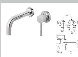
2 hole basin mixer single lever wall mounted with water flow straightener with water flow aerator ceramic cartridge CAR-K35B 2 x 1/2" inlets 1 x 1/2" outlet min-max wall mount 53-73mm for the valve minimum operating pressure 0.2 bar LP
