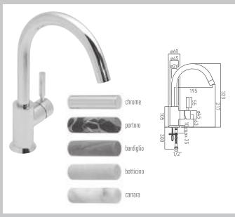
origins mono sink mixer single lever deck mounted with swivel spout with water flow straightener with water flow aerator ceramic cartridge CAR-K35B 2 x 1/2" nut x 400mm flexipipe connections deck mount drill hole diameter 33mm minimum operating pressure 0.2 bar LP
