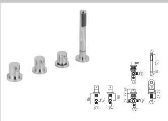
4 hole bath shower mixer deck mounted without spout for use with bath filler waste and overflow cold ceramic cartridge ELE-VALVE/CD-3/4-CL hot ceramic cartridge ELE-VALVE/CD-3/4-HT 2 x 3/4" x 3/4" x 500mm flexipipe connections valve deck mount drill hole diameter 33mm diverter deck mount drill hole diameter 46mm handset deck mount drill hole diameter 27mm minimum operating pressure 1.0 bar MP
