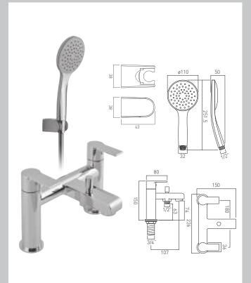
2 hole bath shower mixer single lever deck mounted with shower kit cold ceramic cartridge ION-VALVE/CD/CL-3/4 hot ceramic cartridge ION-VALVE/CD/HT-3/4 2 x 3/4" fitted tails deck mount drill hole diameter 28-30mm minimum operating pressure 0.2 bar LP
