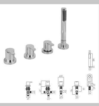
4 hole bath shower mixer deck mounted with shower kit without spout for use with bath filler waste and overflow ceramic cartridge ELE-DIVERTER/D-CART 2 x 3/4" x 3/4" x 500mm flexipipe connections valve deck mount drill hole diameter 33mm diverter deck mount drill hole 2 diameter 7mm minimum operating pressure 1.0 bar MP
